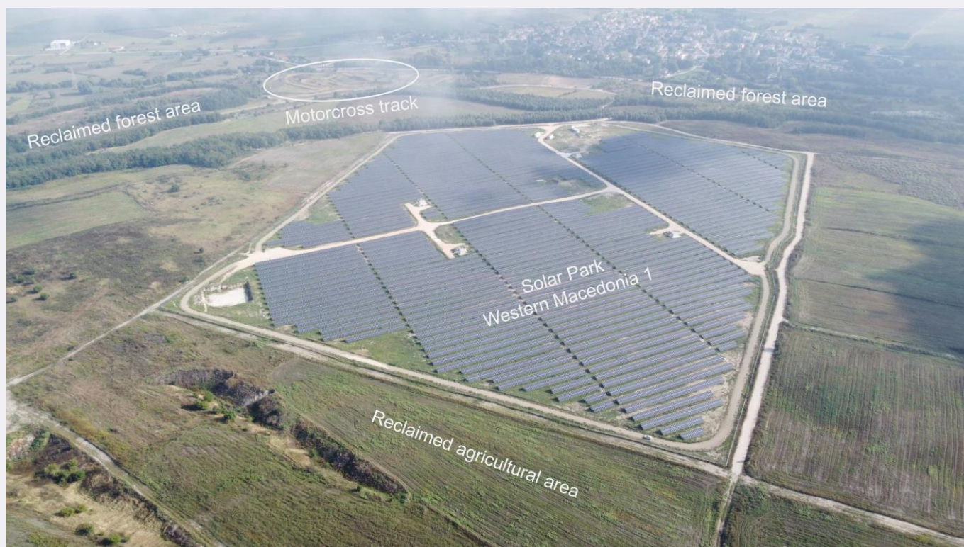
Land restoration and a 15 MW solar PV park near Ptolemais at the West Macedonia Lignite Centre – part of the 550 MW Kozani solar project
