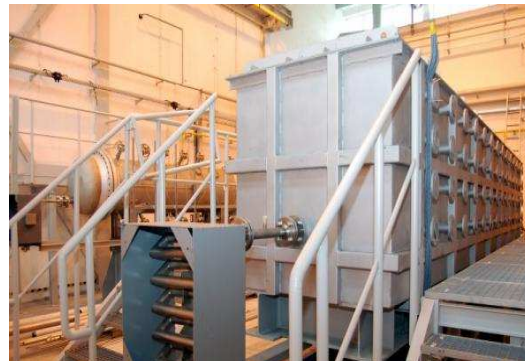
A non-pressure reactor for simulating the underground coal gasification process
